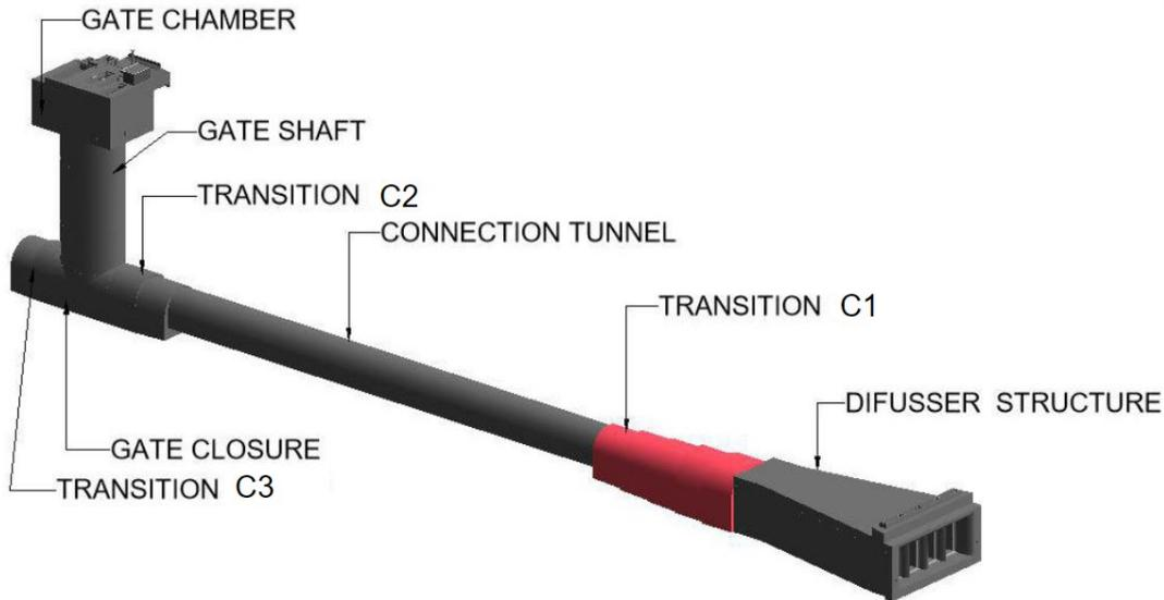
**Figure 2 – 3D view of Transitions and Connection Tunnel between Gate Shaft and Tantangara Intake (Diffuser)**
