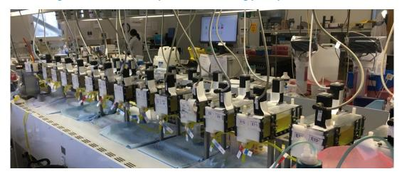
Figure 1: Arafura's NdPr separation circuit during pilot operation at ANSTO
