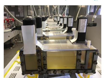
Figure 2: Side on view of SX mixer-settlers in the NdPr separation circuit during pilot operation
