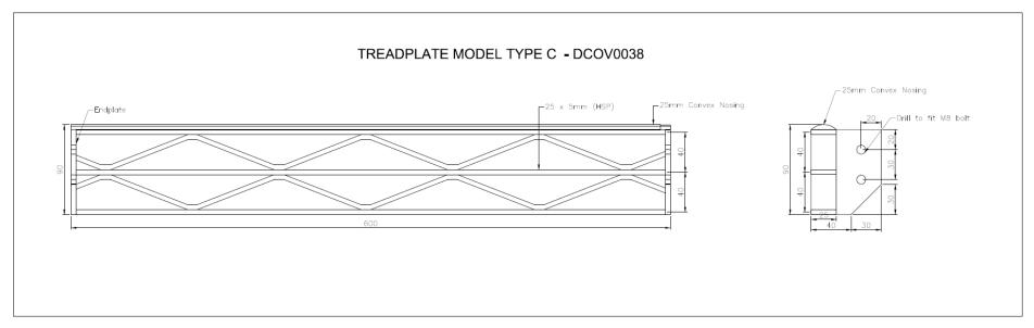
Fig 3: Diamond Treadplate Model Type C - BAE Part No. DCOV0038
